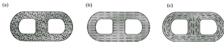
FIGURE 14.3 A part made by three different processes, showing grain flow. (a) casting, (b) machining, (c) forging. Source: Forging industry Association.
